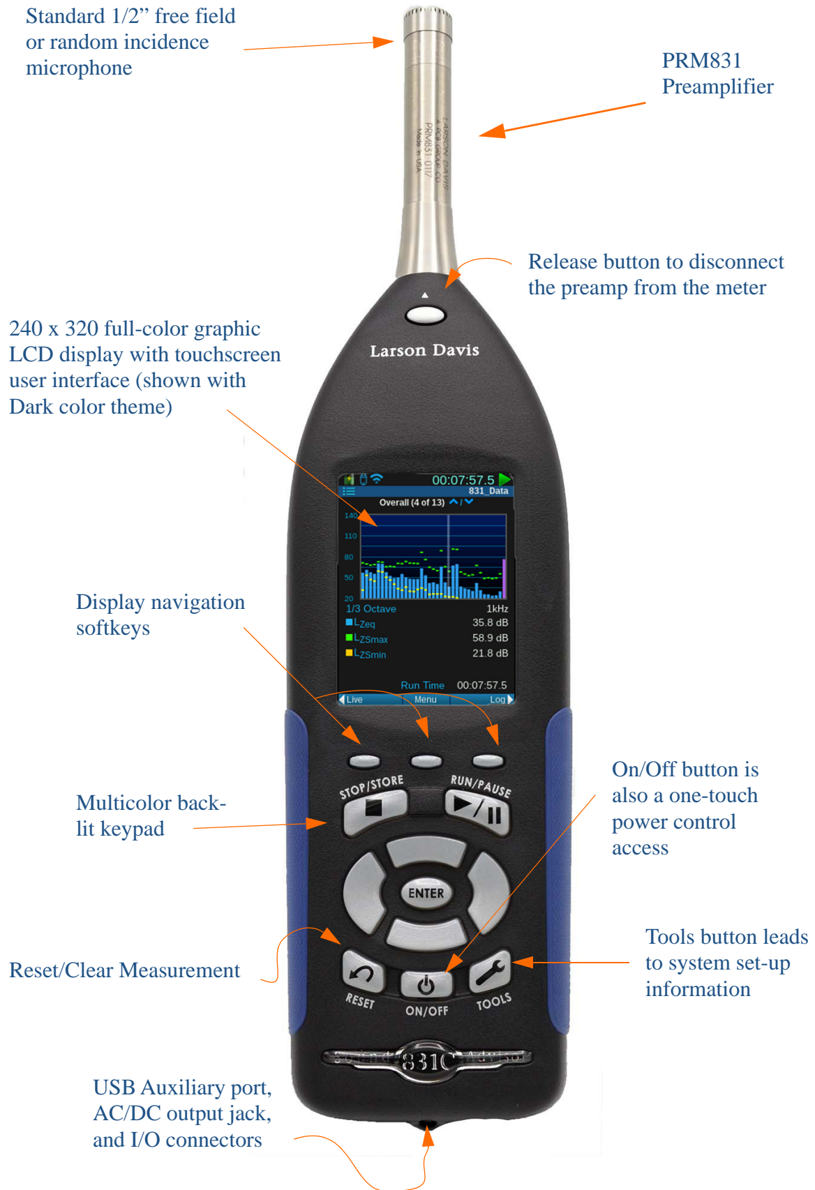
FIGURE 2-1 SoundAdvisor Instrument Overview (front)
