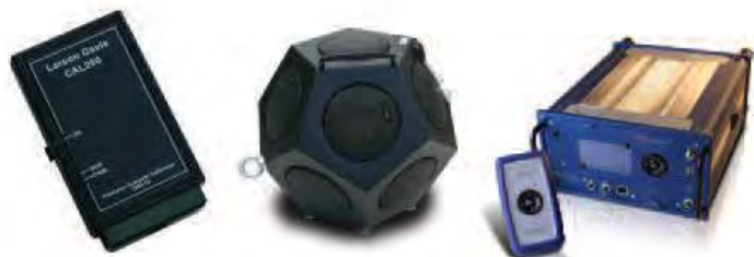
CAL200 1 kHz, 94 and 114 dB, Calibrator
